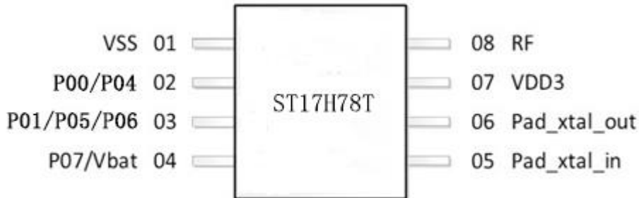
Figure 1: Pin Assignment – ST17H78T SOP8 package
